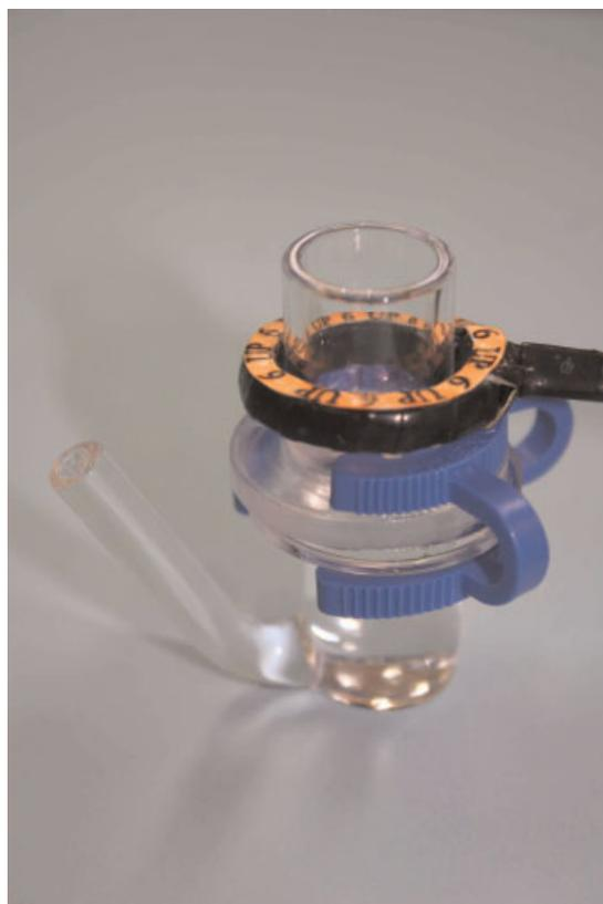
**Figure 3.** *In vitro* diffusion cell with PEMF-Dermaportation coil applied to the exterior of the cell.
