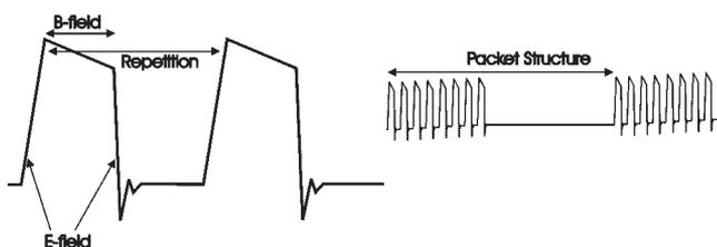
**Figure 2.** Schematic of a PEMF-Dermaportation waveform.
